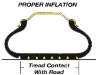
*The correct profile for full contact with the road which results in minimum tire performance is shown above. Because radial ply tires have a characteristic buldge in the sidewall even when properly inflated, it is impossible to visually determine the degree of inflation. Use a reliable air guige to check the inflation pressure.*
